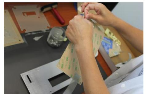
out as to prevent any air from being trapped under the membrane switch. The adhesives are pressure sensitive and firm pressure is required to insure a strong bond. Please take note that dirt and air must not stay trapped under the membrane switch (it may cause the circuit to be constantly closed). We recommend flexing the unit no more than .25" of flex per 4" of unit length flex of the unit during assembly.
