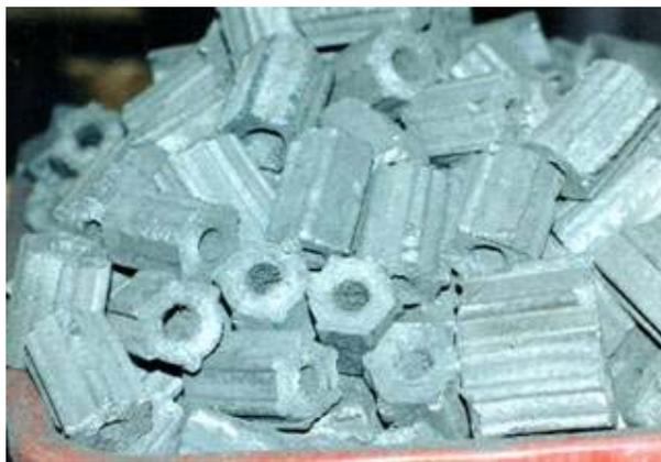
Figure 2. Bamboo briquette charcoal
