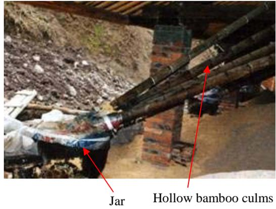
Figure 11 the instrument for condensing smoke and colleting crude bamboo vinegar.
