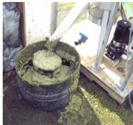
The green sludge of algae and phosphorus separated from the Waihi oxidation pond effluent.
