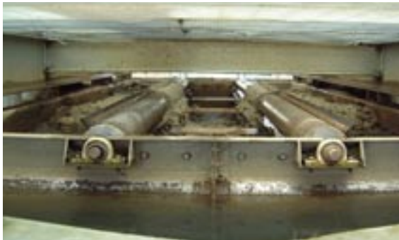
Algae and phosphorus sludge separated from municipal wastewater treatment plant treated effluent.
