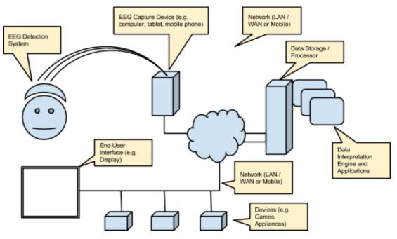
Figure 1: Diagrammatic Representation of EEG System
