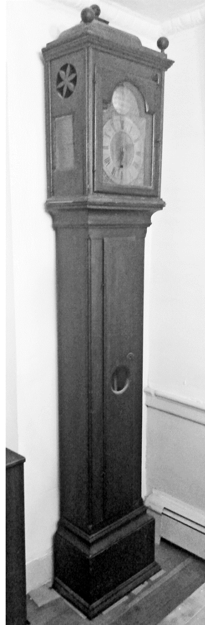
The clock movement is housed in its original Amesbury tall case, likely made by Samuel Blasdel (1717-1769). The width of the case was dictated by the swing of the long pendulum, and the height by the drop of the weight needed to power the clock for 30 hours.
