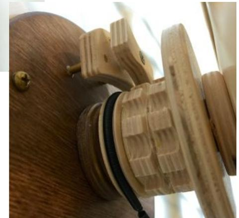
Image 3 Right -This shows the belt in the correct position over the pulley of the upper patterning wheel.
