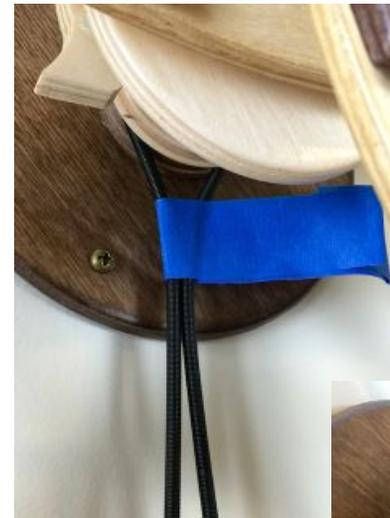
Image 2 Left -This shows how the belt is tape in place hanging from the back pulley. Do not remove tape until instructed to do so in steps.
