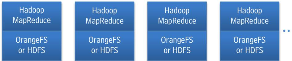
The tests were performed on 8 Dell PowerEdge R720s with Local SSDs for metadata and 12 2-TB drives for data. For the first test (above), MapReduce was run over OrangeFS and HDFS locally on the same nodes. The nodes were interconnected with 10Gb/s Ethernet.
