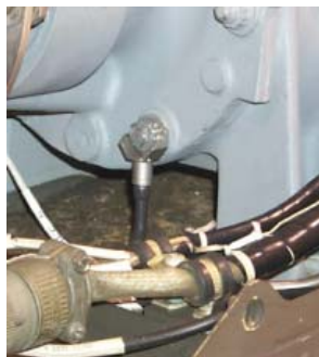
Figure 2 - VMEP Bracket-sensor on UH60 Gearbox
