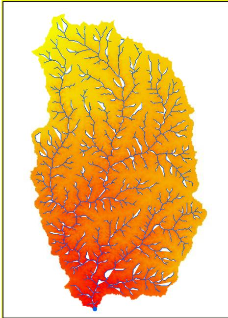
**Figure 20. Flow Accumulation Network. Solid blue lines indicate the location of stream channels in the surface-water model, delineated based on the digital elevation model.**
