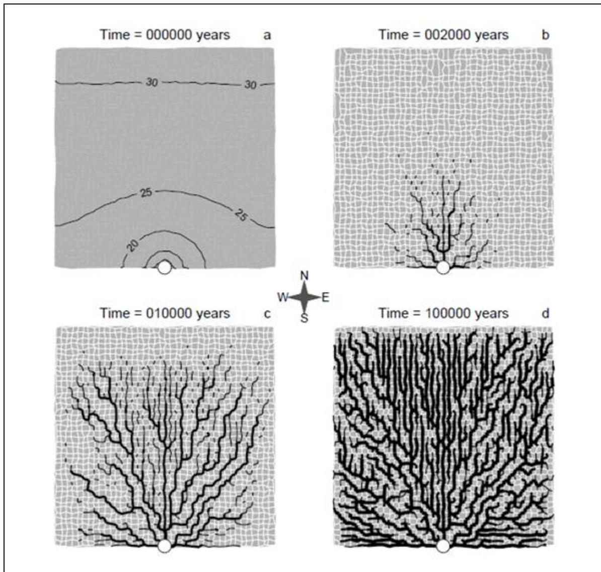
Figure 17. Conduit development simulated for a medium with uniform distributed recharge and uniform hydraulic boundaries (Kaufman, 2005).
