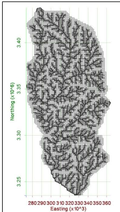
**Figure 19. Plan view of MODFLOW-USG quadtree grid. Note the full discretization of the dense stream network.**
