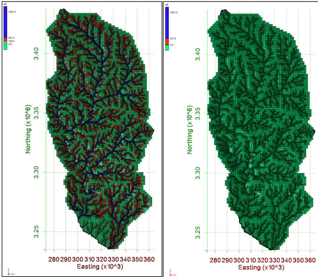
**Figure 22. Hydraulic Conductivity field for layer 1(left) and layer 2 (right). Note the higher conductivity of the stream channels to simulate conduit flow in layer 1.**
