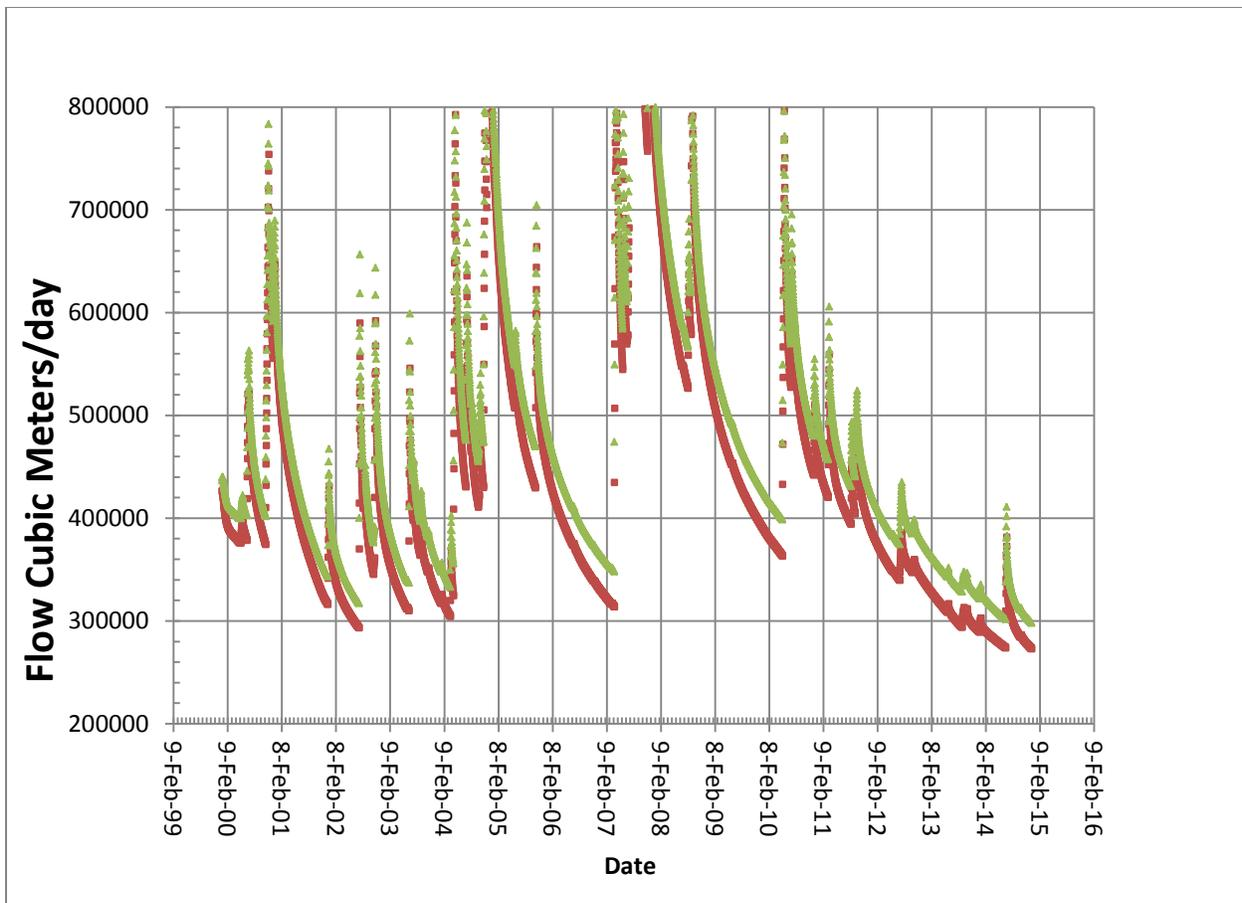
**Figure 26. Modeled baseflow for a scenario where 8,000 gpm of groundwater is exported from Juno (red squares) compared to a simulation without groundwater export (green triangles).**
