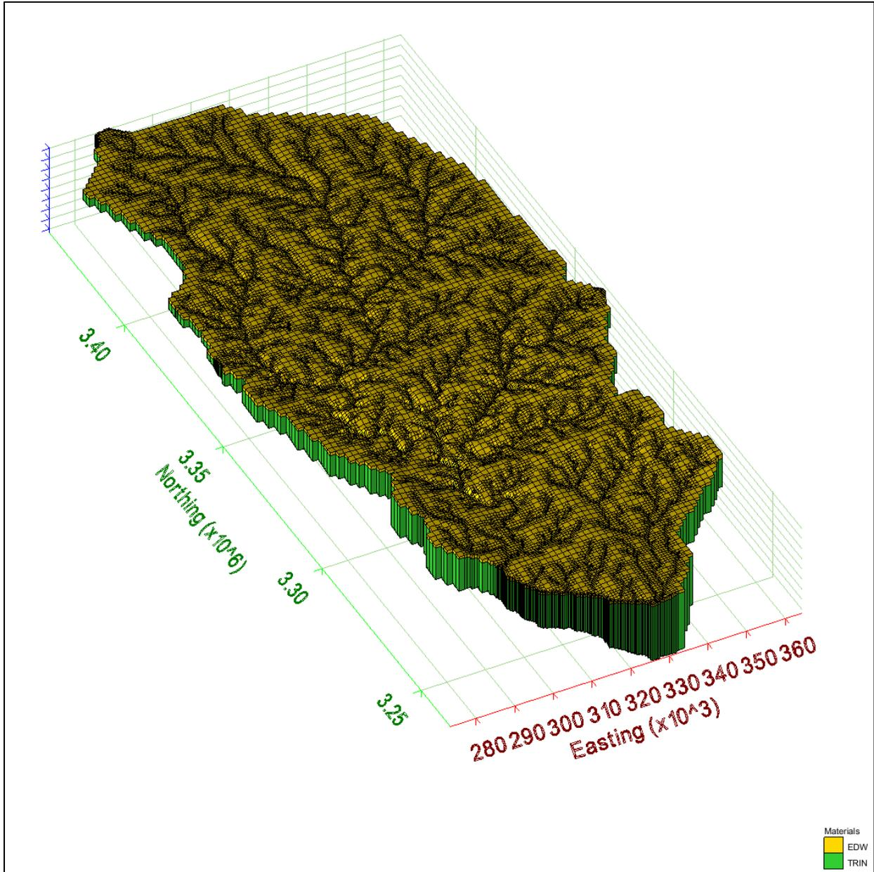
Figure 21. Oblique view of the refined groundwater-flow model.
