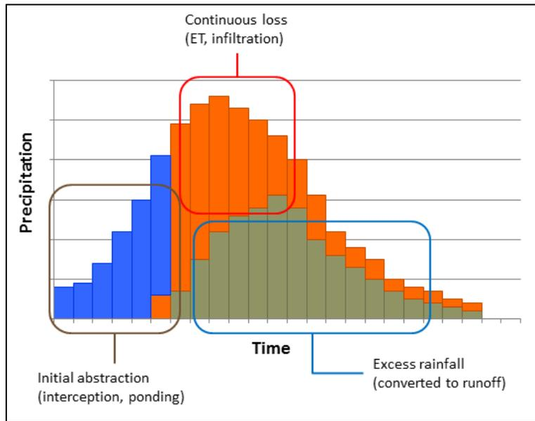
**Figure 9. Illustration of loss method applied to precipitation hyetograph.**
