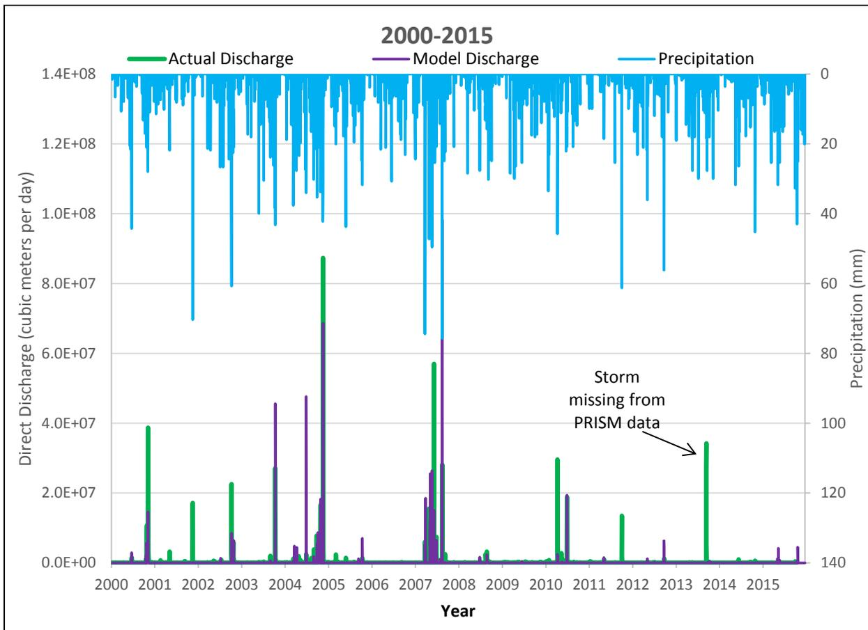
**Figure 16. Results of direct runoff calculations in the long-term surface-water model.**
