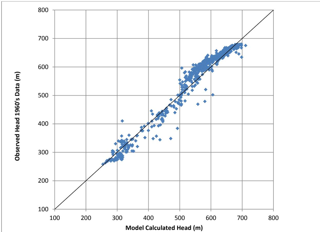
**Figure 23. Steady-State Calibration plot of observed heads versus modeled heads. A perfect fit is when every point falls on the X-Y line shown in the plot.**
