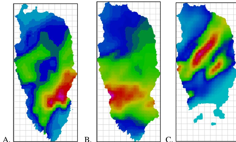
**Figure 13. Examples of pixelated NEXRAD precipitation data illustrating the high degree of spatial variability in precipitation intensity for three days in 2007. Rainfall intensity is depicted ranging from low (blue) to high (red and pink). (A) June 11, 2007. Maximum rainfall 5 cm [2 inches]. (B.) May 1, 2007. Maximum rainfall 11.5 cm [4.5 inches]. (C.) August 17, 2007. Maximum rainfall 25 cm [10 inches].**
