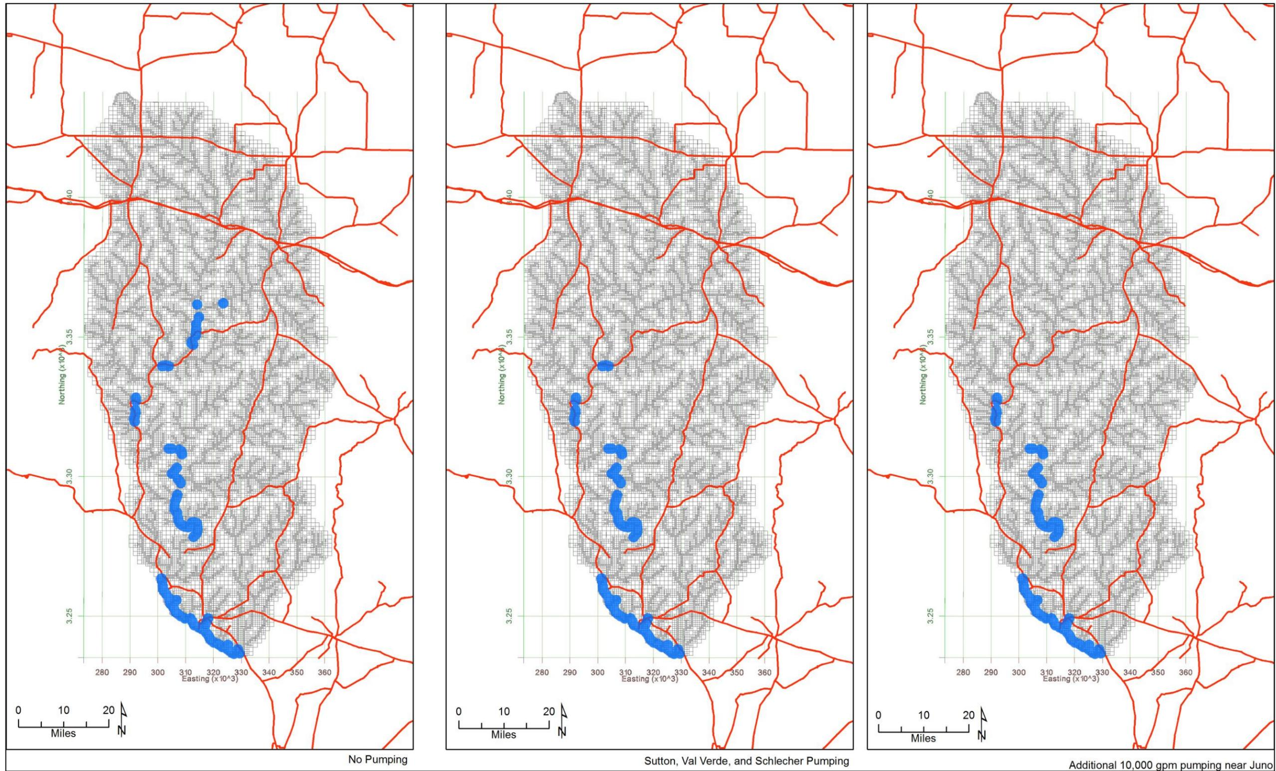
**Figure 25. Model predicted spring locations. From left to right: Spring locations with no pumping, pumping as estimated by the Texas Water Development Board in Sutton, Val Verde, and Schlecher Counties, and additional pumping for export from a well field near Juno. Blue marker symbols are predicted spring locations.**
