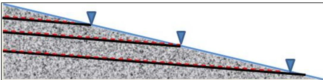
**Figure 2. Schematic of hypothesized intersection of preferential flow paths with riverbed at locations where the riverbed incises into the lower stratigraphic units. Black lines denote stratigraphic unit surfaces. Blue line denotes riverbed surface. Red dashed lines denote preferential flow path development along stratigraphic surfaces. Inverted triangles denote spring locations in riverbed. [Not to scale, vertical dimension exaggerated.]**
