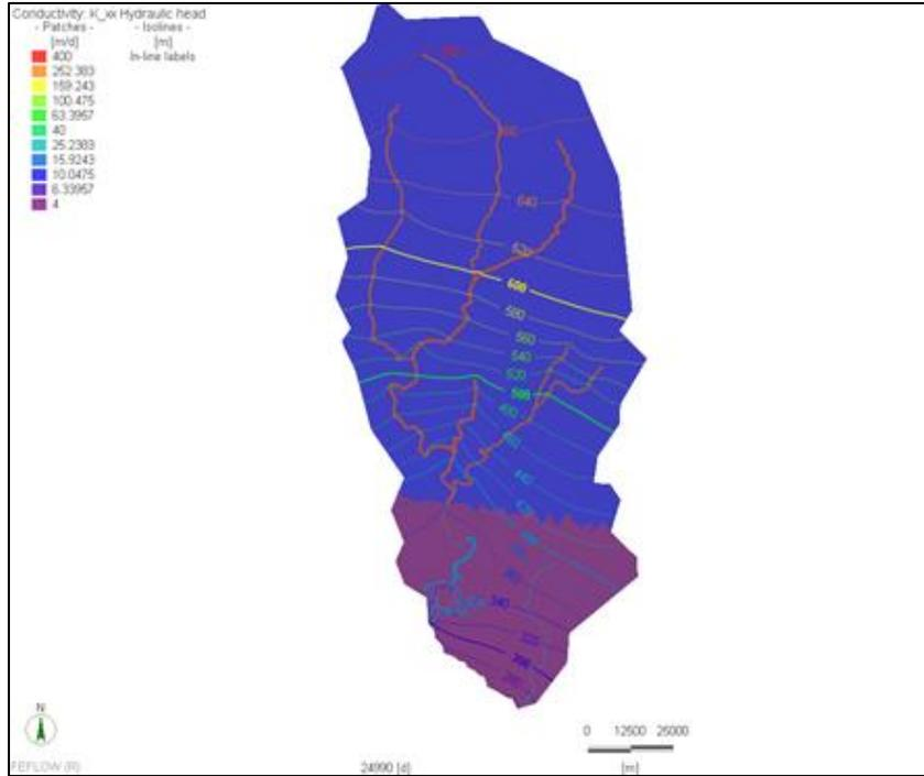
**Figure 18. 2015 Finite Element Model Conduits. Solid lines denote the location and extent of discrete features aligned with the major river channels in the groundwater flow model (Green et al., 2015)**
