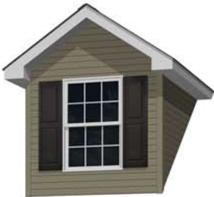
7' Doghouse Dormer for a 9/12 Pitch Roof with a 3046 Window and Shutters
