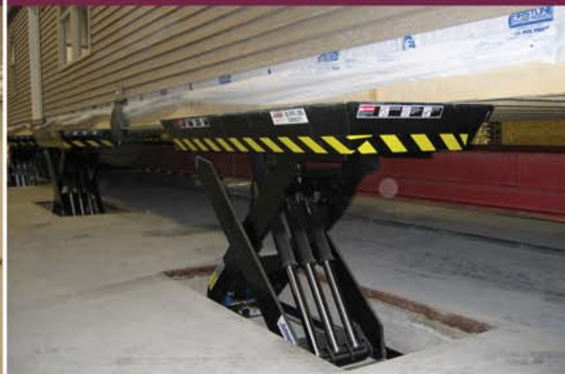
Each model is lifted within one quarter-inch of level by eight independent hydraulic lifts and gently set on a heavy-duty transport carrier.
