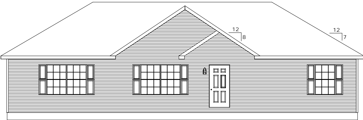
27'-5" x 56' RICHMOND Model (7/12 Hip Roof) Shown with Optional Reverse Gable Dormer with Return Eave
