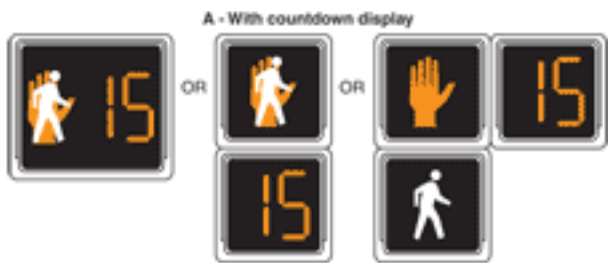
Figure 4E-1. Typical Pedestrian Signal Indications
