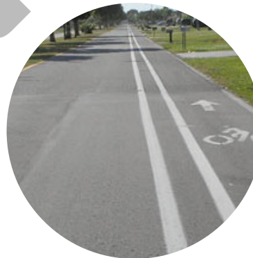
Buffered bike lane in a residential area of Cape Coral, FL, where simple solid white lines are used when the buffer zone is less than three feet wide. source: NACTO
