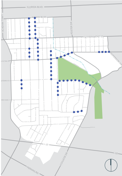
Observed drainage issues
