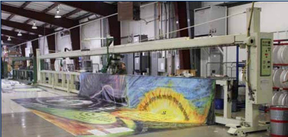
Hot Air Welding
