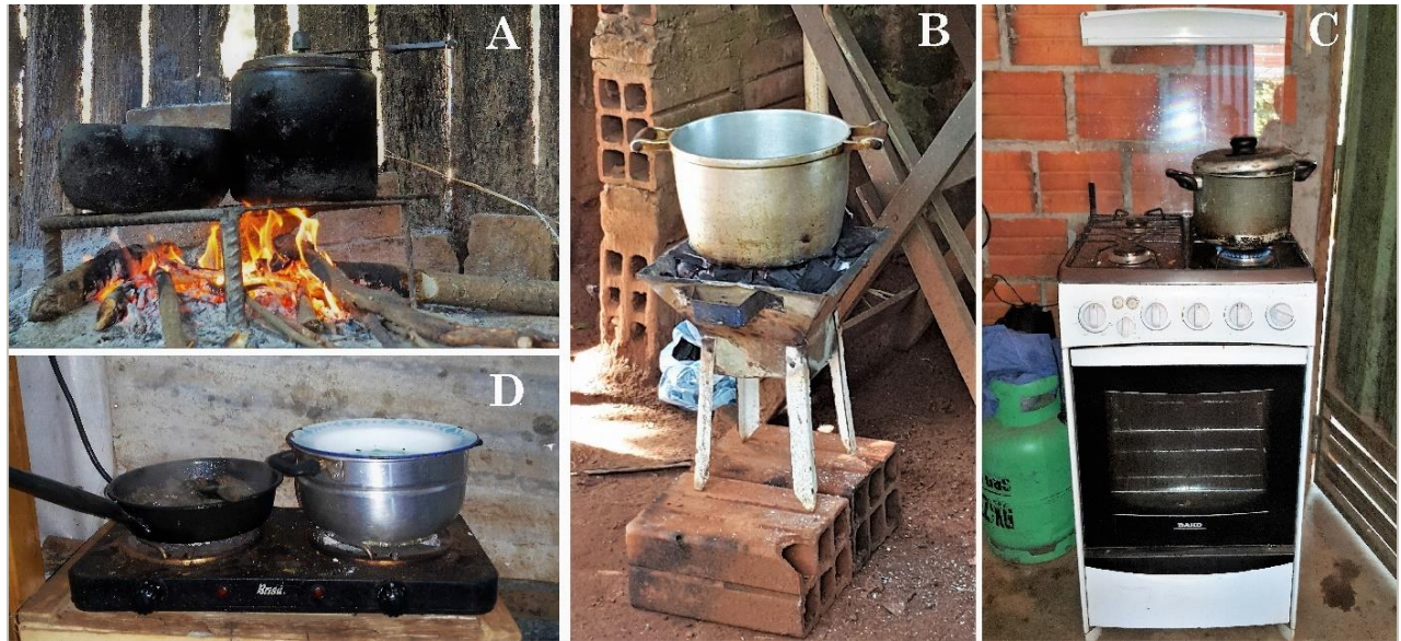
Figure 9. Cookstoves commonly found in the sub-urban and rural village. A: Open fire (firewood). B: Brazier (charcoal). C: LPG Cookstove. D: Hot plate (electric).
