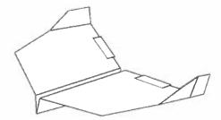
This plane is an excellent outdoor glider. Launch straight up and it will glide down in big lazy circles. Adjust the elevator on the back edge of the wing to perfect the flight characteristics.
