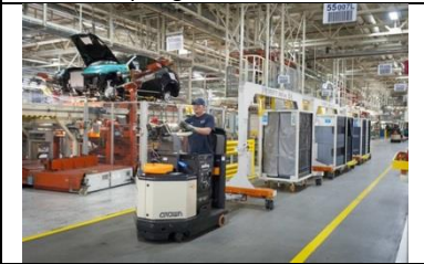
Fuel cell powered materials handling equipment at BMW Manufacturing Plant – Greer, South Carolina
