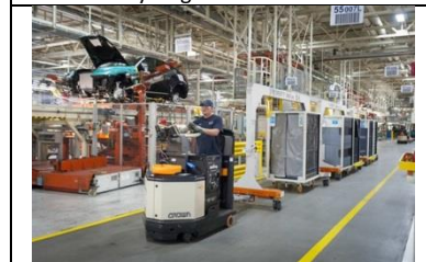
Fuel cell powered material handling equipment at BMW Manufacturing Plant – Greer, South Carolina
