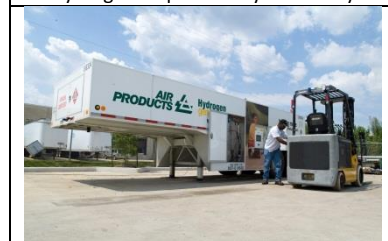
Mobile Hydrogen Fueler and Forklift
