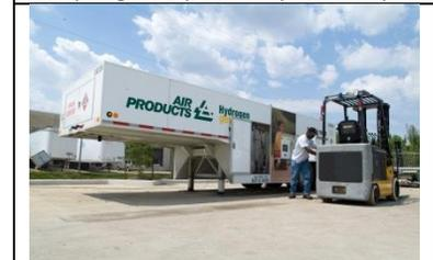
Mobile Hydrogen Fueller and Forklift
