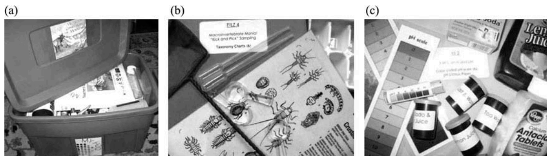
Figure 1. Images representing the My H 2 O kit materials and supplies, which include (a) the My H 2 O Curriculum Guide and My Water Comes from the Mountains book as well as other age-appropriate literature, music and video resources; (b) benthic macroinvertebrate identification keys, pipettes, hand lenses, specimen tray and dip net for animal-based water quality assessments and (c) supplies for pH studies including lemon juice, antacids, baking soda, litmus paper and pH scales. Also included (not shown) is a 3-D relief map of the local watershed.
