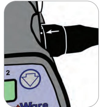
Figure 10: Correct Locking Position
