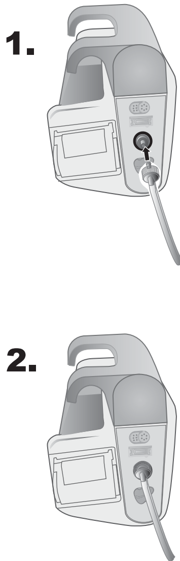
Figure 8-1 Attaching a Dual Lumen Hose to the X Series Unit
