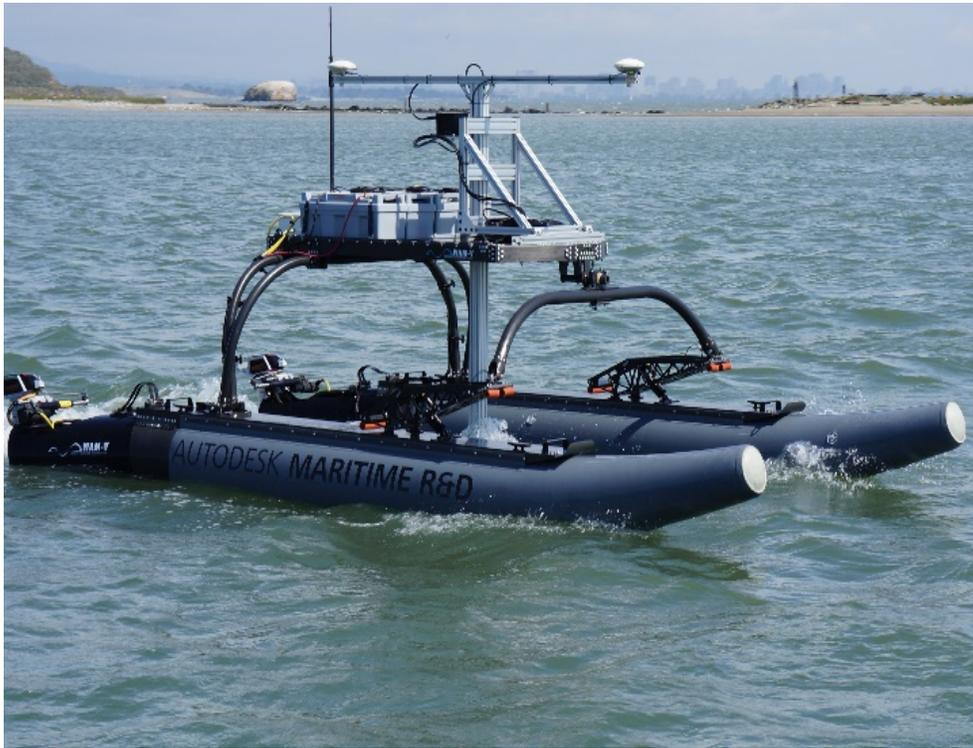
The WAM-V 16' B.O.S.S. (Benthic Operations Survey System) are unmanned, robotic surface vessels specifically equipped for bathymetric data collection
