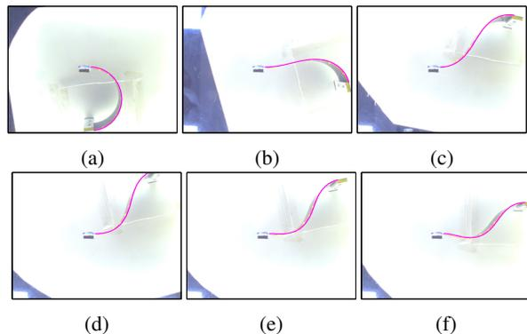
Fig. 6: Tracking the shape of a deformed elastic rod. Magenta curves are produced using our state estimation procedure.
