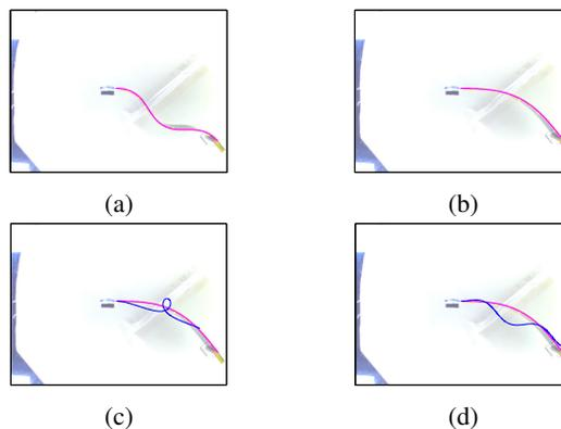
Fig. 8: Tracking the shape of an elastic rod before (a) and after (b) an instability. The estimation procedure sometimes converges to a local minima of the error, as shown by the blue curves in (c) and (d).
