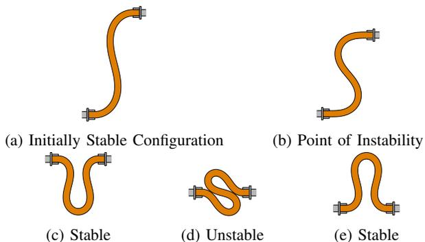
Fig. 2: An elastic rod passing through a bifurcation.
