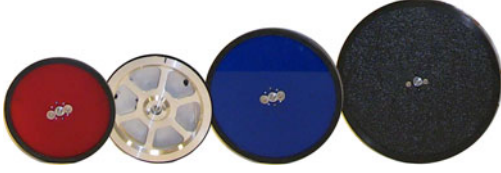
Fig. 7. Four wheel sizes used for experimental validation. These wheels are 10.16, 10.48, 12.7, and 15.24 cm in diameter.
