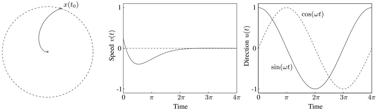
Fig. 2. The optimal path  $x(t)$  and speed  $v(t)$  given the direction  $u(t)$  to reach the origin when  $t_0 = 0$  and  $q = r = 1$  for  $\omega = 0.5$ .
