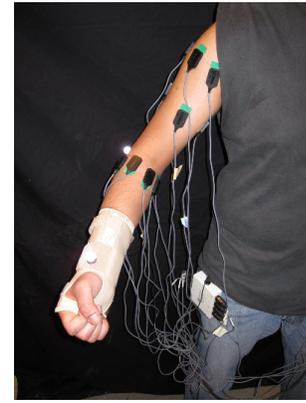
Fig. 2. Placement of EMG electrodes on subject.
