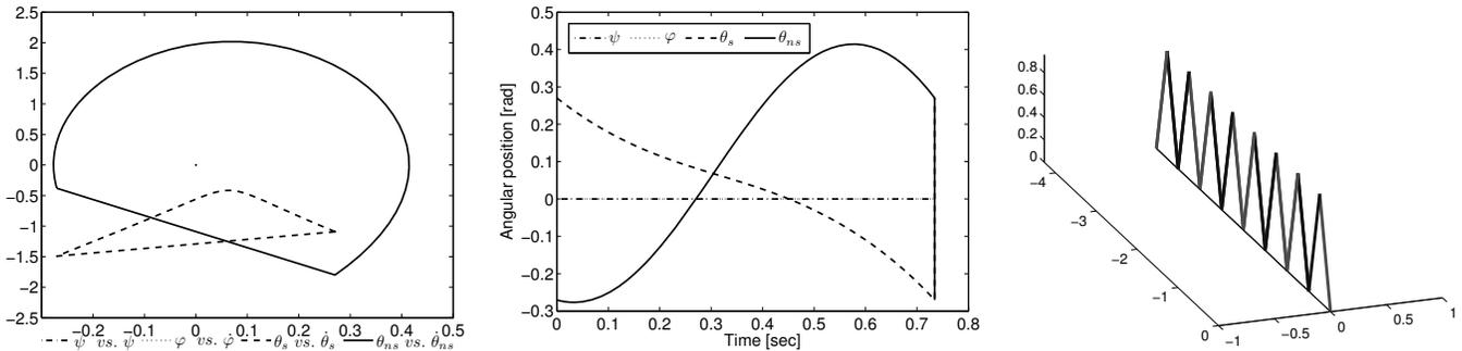
Fig. 3. Straight-ahead 1-step gait: phase portrait (left), coordinate trajectories (center), and multi-step visualization (right). The phase portrait shows planar slices of  $\mathcal{O}_{4D}^t$  by plotting angular positions against angular velocities, which we use to illustrate 1-step periodicity in phase space.
