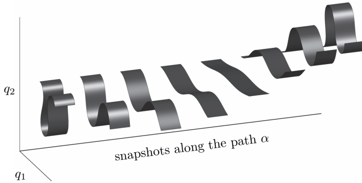
FIG. 3. A sequence of configurations of a planar elastica corresponding to the path \alpha in Figure 4a. The leftmost and rightmost configurations are local solutions of (7.1), i.e., they are stable equilibrium configurations. The six intermediate configurations are not local minima of (7.1) and are therefore unstable equilibrium configurations.
