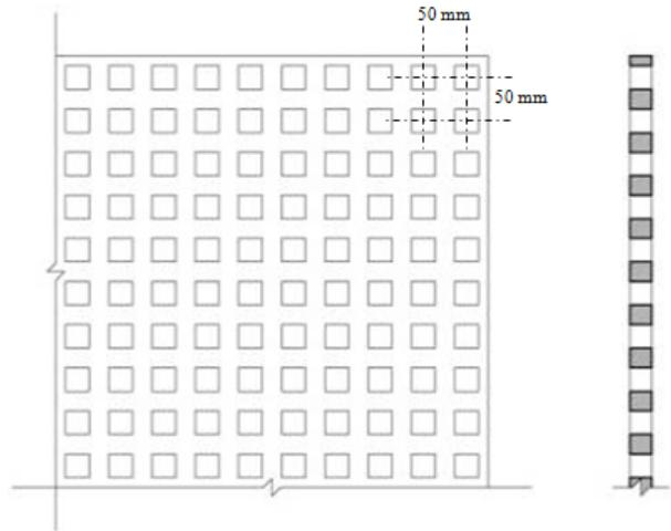
Fig. 2. Example Solar Screen 30% Elevation and Section
