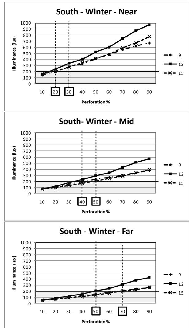
Fig. 4. Illuminance against perforation % for the Winter season, with a highlight on the suitable perforation for the tested times in the South orientation.
