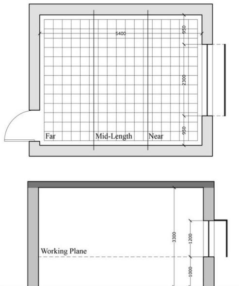
Fig. 1. Assumed design parameters of the analyzed indoor space.
