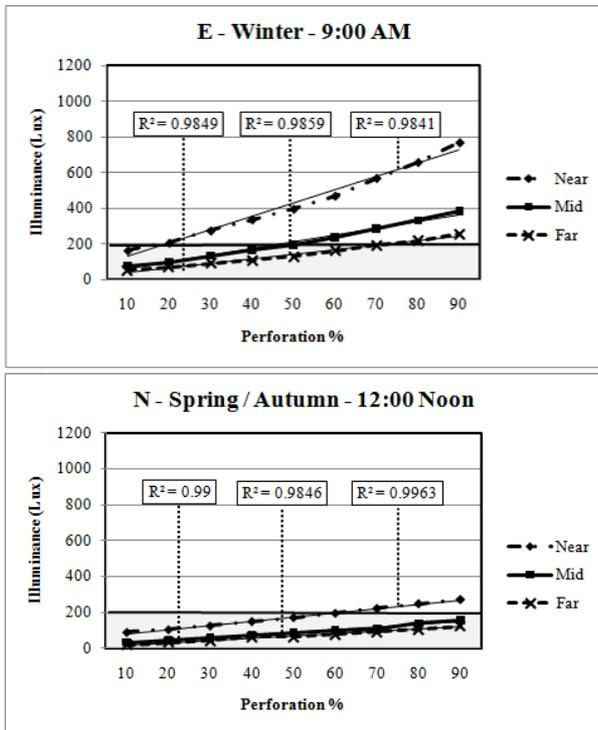
Fig. 3. Solar screen perforation percentage against illuminance values showing linear performance.
