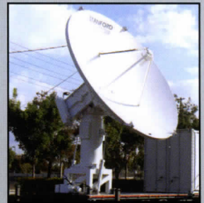
PG-2506 Transportable Ground Station (TGS)
