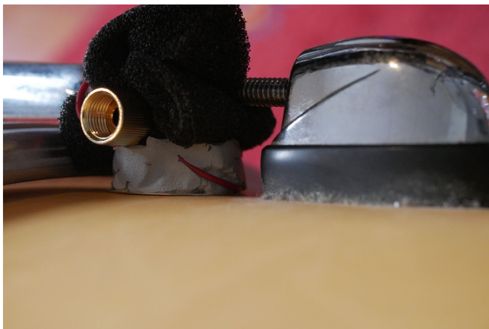
A hand-made contact microphone was fixed to the shell in order to create the click samples.
