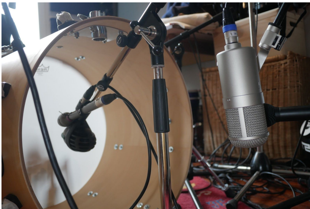
EV RE15, AKG D112 inside the bass drum, Neumann U47fet and Beyer M88 in front.
