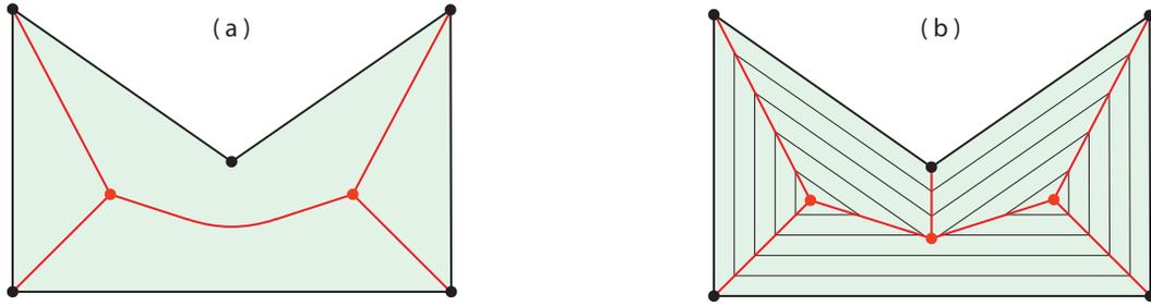
FIGURE 1. (a) Medial axis and (b) straight skeleton.
