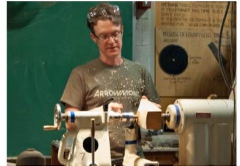
Mark uses a 1/2 inch bowl gouge and a pulling cut to form the underside shape. Pulling and using 1/3 of the wing makes interrupted cuts easy.
