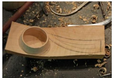
Now comes the fun part—shaping! Here is one of his iconic designs ready to be taken to the band saw for the rough cuts. A lot of hand work with sharp chisels is then required to make the spoon on Page 1.
