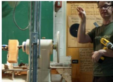
A disc of good grade of plywood is put on the outboard side of the lathe with a face plate. Weights attached to this plate counterbalance the stock between centers.
