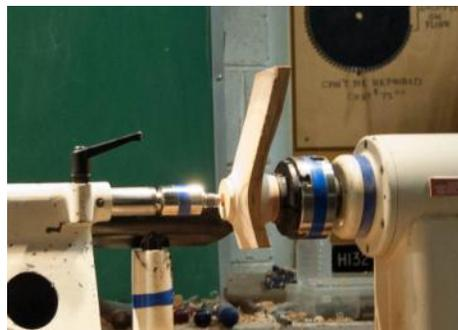
Once the proper depth has been achieved for the bowl it can be sanded in the inside—carefully! Using a jam chuck in the jaws, he then shapes the base to conform to the top curve and removes the tenon.
