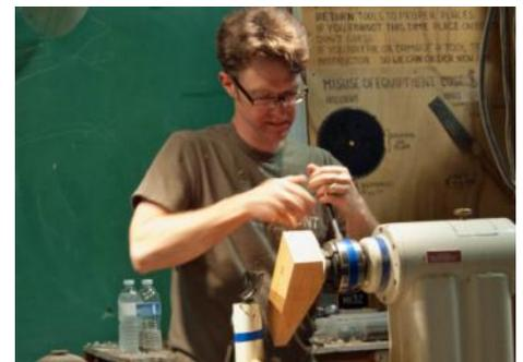
The piece is reversed and put in a 4-jaw chuck. The tenon is carefully made with a slight dovetail shape so as to pull the piece into the jaws.
