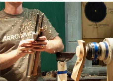
After shaping the top side of the handle and the outside of the bowl, Mark turns his attention to the inside of the bowl. A more shallow grind is needed to cleanly cut the inside of the bowl.
