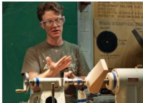
Here the tenon is completed. It was formed first with a bowl gouge and then the edges were refined with a 3/8ths spindle gouge.
