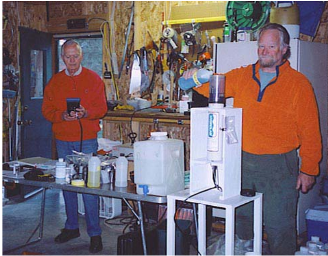
Meet early to calibrate the water-quality sonde, which is checked for the accuracy of pH, specific conductance, temperature, and dissolved oxygen readings.
