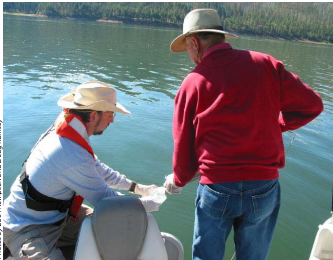
Water samples are collected at the bottom and top of the lake using a point-sampler on a rope with a weighted "messenger" to trigger open the sampler. Samples are poured into one-liter cube bottles. A sample number with a suffix of "L" indicates the lower sample, and a "U" indicates the upper sample.
