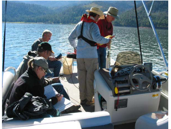
The sonde is lowered into the lake 5 or 10 feet at a time, and water properties are sent to the data unit, where readings are recorded by a notetaker. On this day, we had the luxury of a pontoon boat. Most sampling days are spent in a small outboard motor boat.
