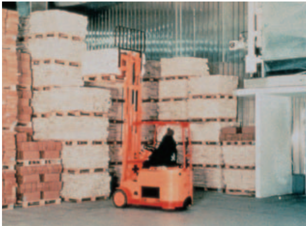
Fig. 14: Forklift truck and heavy storage goods strain the heat-insulated floor of the cold-storage warehouse.
