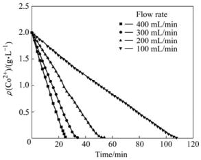
**Fig.5** Co<sup>2+</sup> concentration in solution with time at different flow rates
