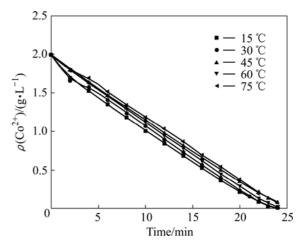
**Fig.3** Co<sup>2+</sup> concentration in solution with time at different temperatures
