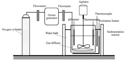
Fig.1 Experimental apparatus
