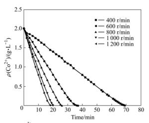
**Fig.2** Co<sup>2+</sup> concentration in solution with time at different stirring speeds
