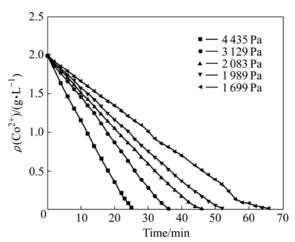
**Fig.4** Co<sup>2+</sup> concentration in solution with time at different ozone partial pressures
