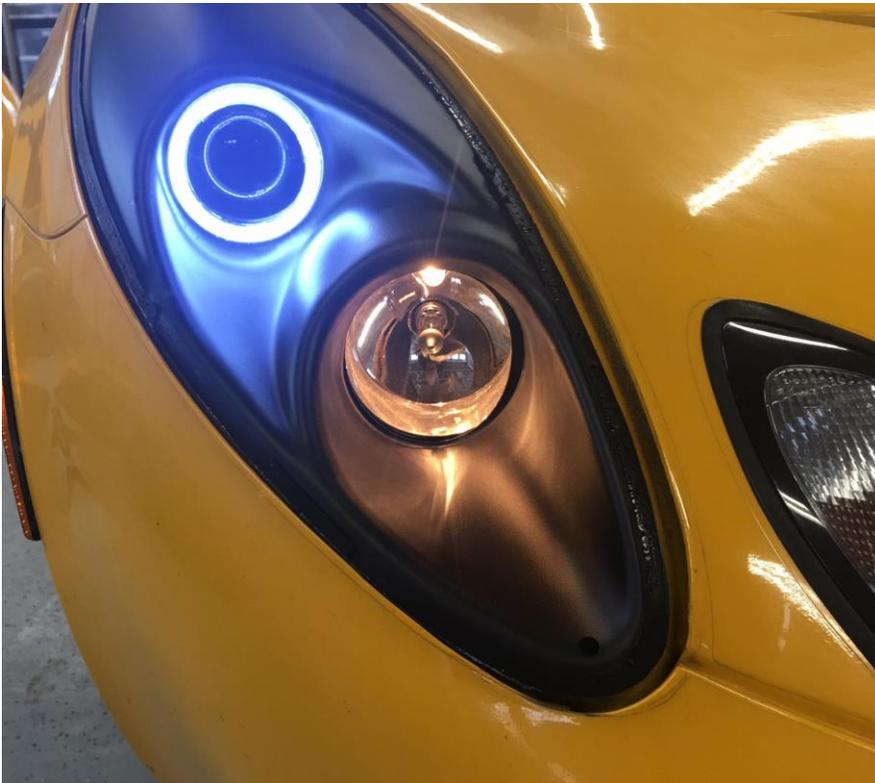
**12. After confirming your halos are functional, remove the housing assembly, reattach the headlight lenses to the housing using a high quality black silicone and reassemble everything in reverse order of removal!**
