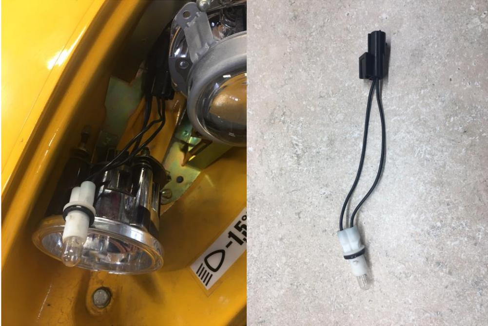
**8. Now using the supplied scotch lock wire taps you can easily tap into the two wires for the parking light. The halos wires can be tapped into either black wire, there is no polarity to worry about. Set up your wire taps and halo wires as pictured and squeeze the metal portion of the wire tap down using a set of pliers. Make sure the metal tap is down as far as it can go, then close the plastic cover down.**
