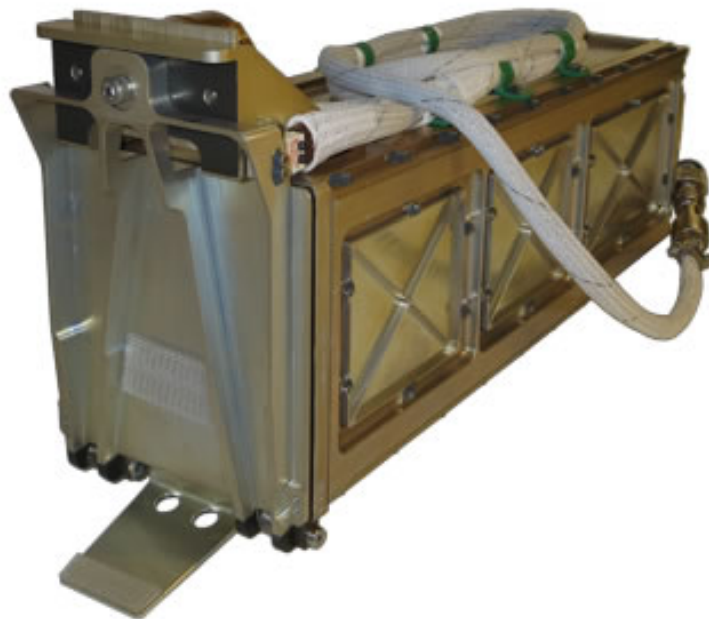
Figure 3: Alodined P-POD Mk. III Rev. E
