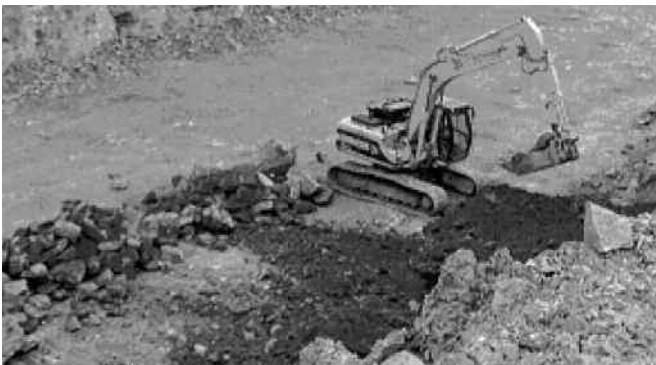
Figure 7. Photograph showing recovery of limestone from contaminated face.
