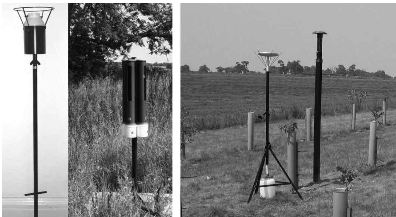
Figure 1. Nuisance dust monitoring methods. From left: Bergerhoff deposition gauge; CERL directional deposition gauge; Frisbee deposition gauge with DustScan directional gauge.
