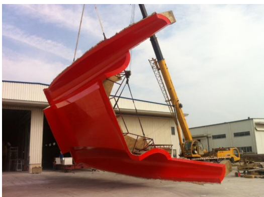
Flipping the hull/bridgedeck mould.
