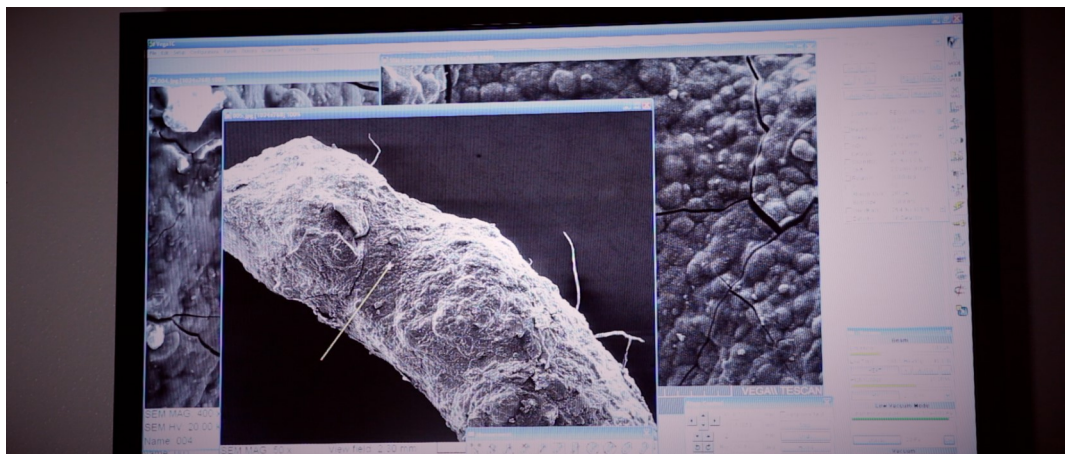
View using Electron Microscope with less magnification showing Carbon Nano Fibers.
