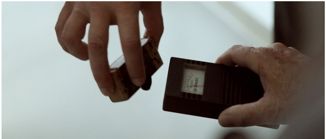
Right: Use of a Gauss meter to measure electromagnetic fields.
