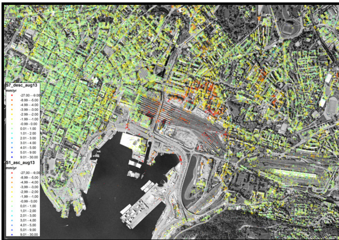
Figure 8: Settling rates measured from satellites with InSAR technology in the Björvika area. Red dots show areas with high settling rates (John Dehls, NGU, August 2013).
