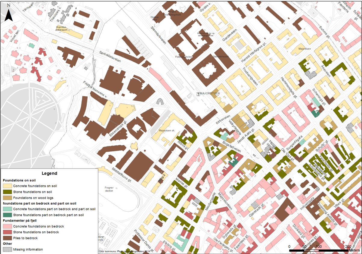
Figure 18; Foundation types relative to the geology that the foundation rests upon in the test area of Majorstuen.
