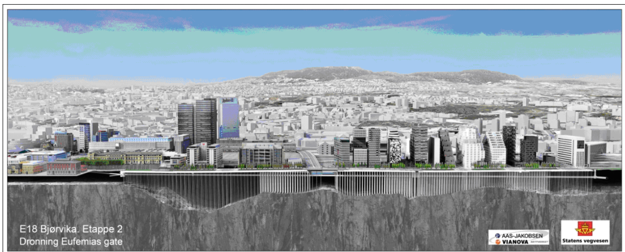
Figure 11: Dronning Eufemias gate in the newly developed area of Bjørvika is more like a bridge than a road. To deal with the deep horizons of clay, often containing a large amount of organic matter, the road is constructed on more than 1000 piles of steel and concrete (Statens Vegvesen).
