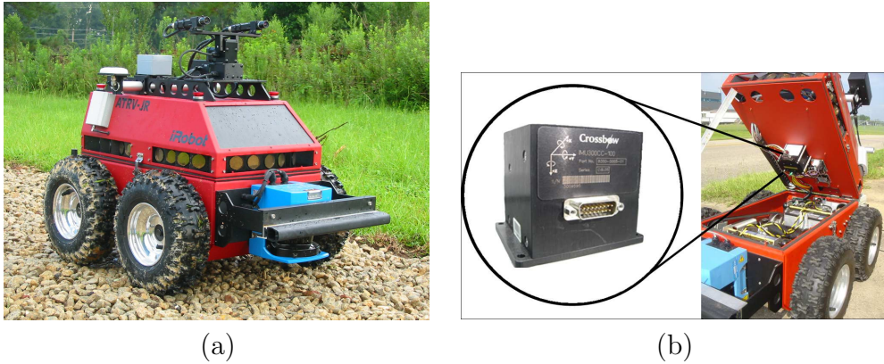
Figure 11: a) The iRobot ATRV-Jr Robot Platform; b) The Mounted Crossbow IMU Sensor
