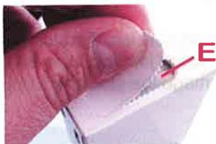
(E) Perforated slide switch access
