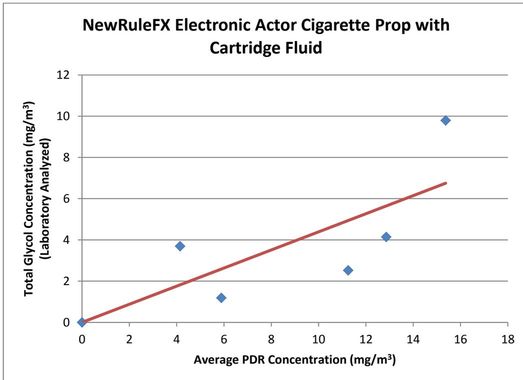
**Figure 1.** Calibration curve for the NewRuleFX Electronic Actor Cigarette Prop with Cartridge Fluid. Calibration factor, based on slope of curve, is  $0.44 \text{ (mg/m}^3 \text{ glycol) / (mg/m}^3 \text{ aerosol)}$ .
