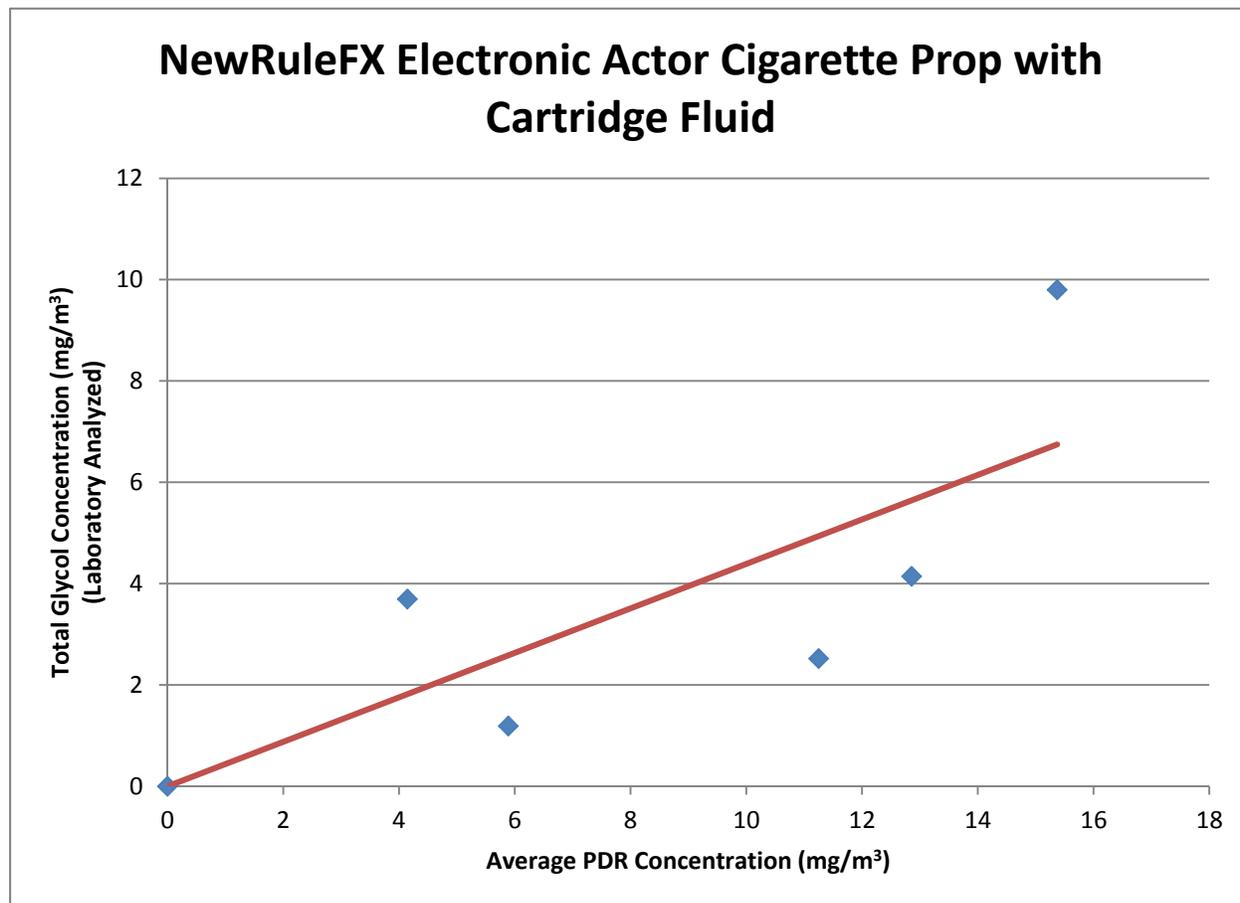
**Figure 1.** Calibration curve for the NewRuleFX Electronic Actor Cigarette Prop with Cartridge Fluid. Calibration factor, based on slope of curve, is 0.44 (mg/m<sup>3</sup> glycol)/ (mg/m<sup>3</sup> aerosol).
