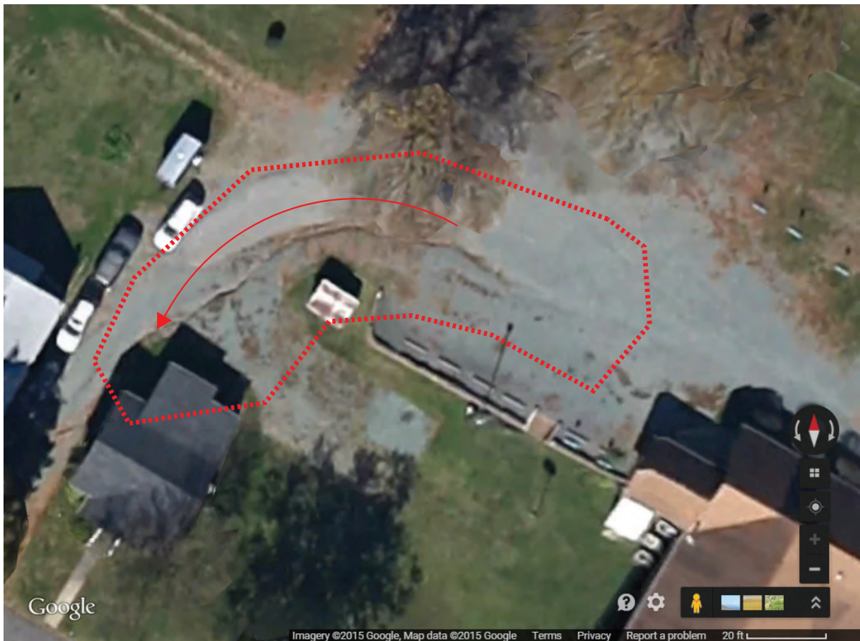
Figure A.2. Google Maps aerial image showing significant gully along stormwater flow path
