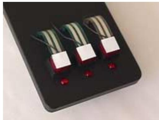
Figure 10: Preview Buttons. This engineering prototype shows buttons retrofit with force sensors, so that a light touch can provide a preview of a button’s behavior – for example fading up an audio track, or gradually enlarging a picture-in-picture.
