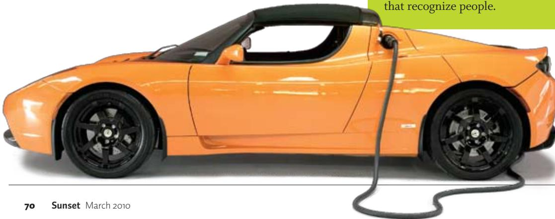
The \$109,000 Tesla Roadster is powered by a 400-volt battery pack and runs at least 200 miles before it needs to be plugged in for a recharge.
