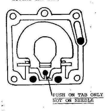
TOP OF FLOAT SHOULD BE PARALLEL WITH TOP OF FLOAT BOWL.
