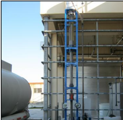
Bench Scale Testing to Determine Optimal Ferric Dose
