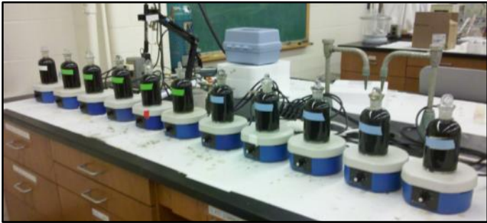
Bench Scale Testing to Determine Optimal Ferric Dose
